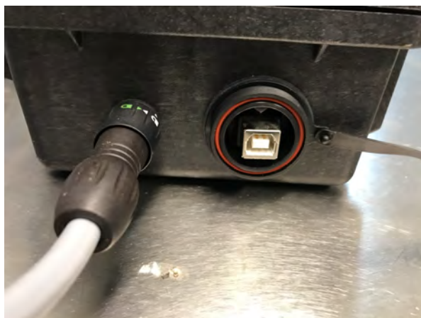
Figure 3: Connections on the PowerCom Box. The sensor cable is connected to the PowerCom Box using the sensor connection to the left. Data are downloaded from the SulfiLogger™ sensor to a computer using the USB port on the right side.
