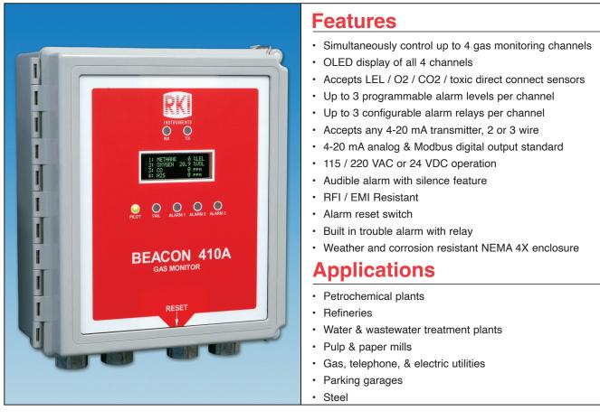
The Beacon 410A is a highly configurable, microprocessor-based, flexible and easy to use 4 channel gas monitoring controller. It simultaneously displays the gas type, readings, and status for four channels of gas detection. It can monitor any combination of direct connect sensors (LEL, O2, CO2, and toxic gas sensors), as well as any 4-20mA transmitter.
